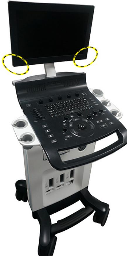
Figure 1-10. Grab the bottom of the monitor
