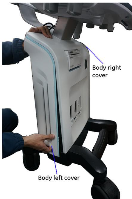
Figure 3-24. Remove the body left cover
