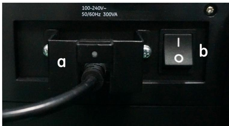
Figure 1-17. Circuit Breaker and Power Plug
