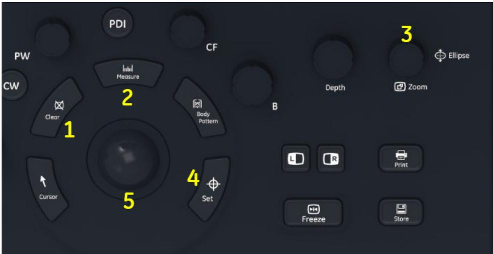
Figure 2-30. Locating Measurement Controls
