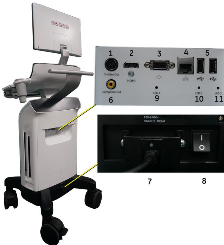
Figure 1-2. Peripheral/Accessory Connector Panel
