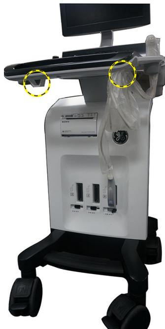
Figure 1-23. Handle probe cable
