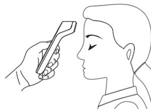
3. Press and release the SCAN button to take a measurement. A double "beep" sound indicates a reading has been taken and displayed on the LCD screen. When a reading is greater than 38.0°C, a warning symbol will flash with Red backlight.
